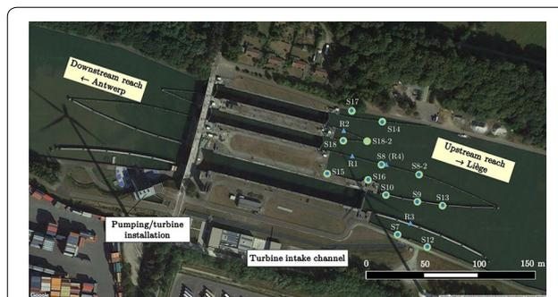
**Fig. 9** Aerial view of the navigation lock complex and receiver array for 2D-positioning in Kwaadmechelen. The green dots are the receivers, the blue dots are the synchronisation tags (collocated with receivers). The blue triangles are reference tags, of which R4 was only installed towards the end of the study, since April 5th 2017. On that day, S8 was also moved to another position, indicated with S8-2. Background from Google Maps Satellite
