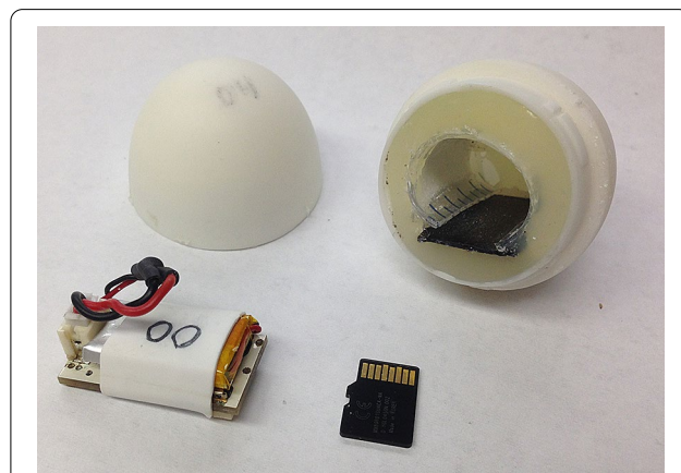
Fig. 1 Photo of artificial egg, data logger, and microSD flash memory card used to measure egg turning behavior and incubation temperatures of snow and Cape petrels. Eggs were made of molded plastic (40 mm breadth × 57 mm length) and both halves were filled with barite powder to add mass to the approximate mass of petrel eggs. Photo by S.A. Shaffer
