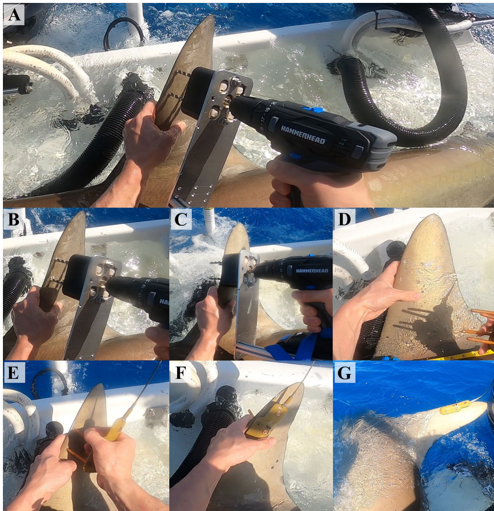
Fig. 7 Photographic time series of the deployment of a SPOT-364 tag on shark 5. The time series shows the A alignment of the drill attachment, B engagement of the drill, C completion of the drilling procedure, D the four simultaneously drilled holes, E alignment of the SPOT-364 tag bolts with the holes, F placement of the SPOT-364 tag before the fastening of the bolts (not shown), and G complete release of shark 5 after 108 s with the SPOT-364 tag tightly fastened toward the top of the first dorsal fin
