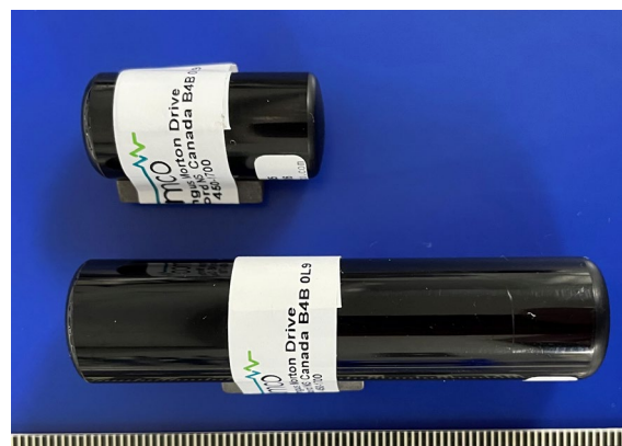
Fig. 1 INNOVASEA V13 (top) and V16 (bottom) acoustic transmitters. These models were surgically implanted subcutaneously in the pre-femoral region of fifteen loggerhead turtles ( Caretta caretta ), with the V13 used for turtles that had straight carapace length (SCL) between 30 and 49 cm, and the V16 used for turtles \geq 50 cm SCL. In this photograph, the inhibitory magnet and adhesive stickers are still attached to the surface of each transmitter. These are removed to activate the transmitter prior to implantation. Scale shows 1 mm increments. Photograph courtesy of Deana Edmunds
